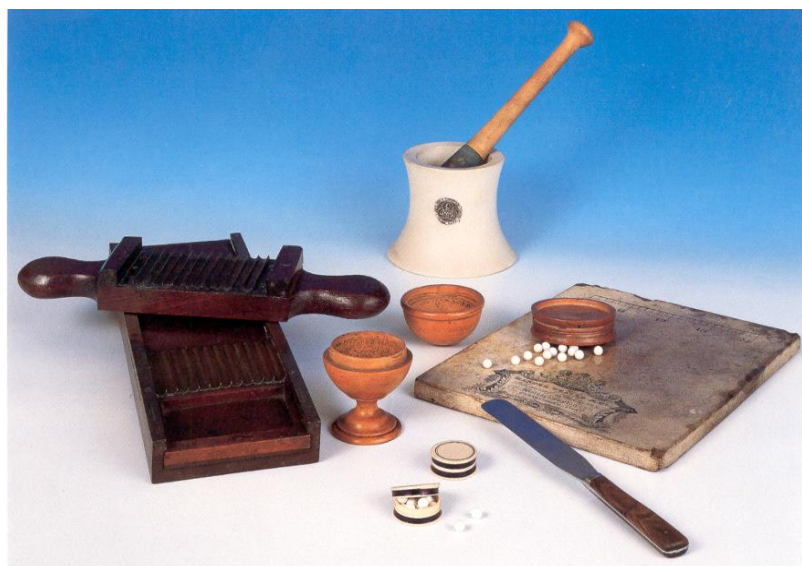
From a Museum postcard showing various apparatus used in pill making. At the back is a, Pill Mortar and Pestle . Centre from left to right, a Pill Machine , Pill Silverer , Pill Tile and Pill Rounder . Front a Pill Box containing pills and a Spatula .
